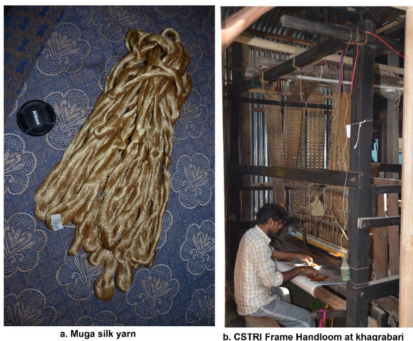
Figure 4. Yarn of muga silk (a) and CSTRI frame handloom at Khagrabari, Coochbehar.
